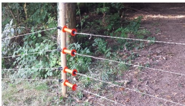
Figure 2: Fix electric wire fence with wooden posts
